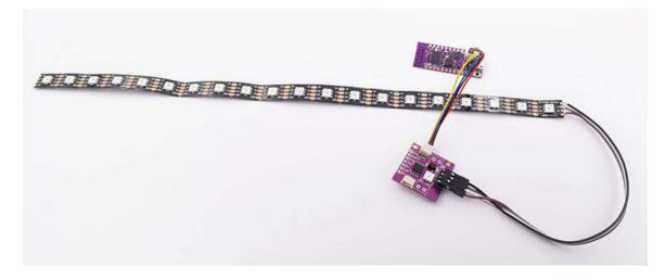
Note: You must use a 5V DC Power supply to power the APA102 LED Strips. Watch the the current consumption when using an LED strips, 5V 4A power supply for 0.5m/ 1m and 5V 10A up to 2m (depending on the application)
